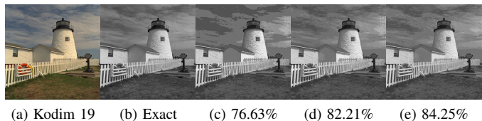
Fig. 20. RGB to Greyscale Conversion of Image 19 in Kodak Dataset:(a) Color Image (b) Exact grayscale Image; Approximate outputs through Outline-3 (c) MAFA-1 (d) MAFA-2 (e) MAFA-3; MSSIM is given with images.
