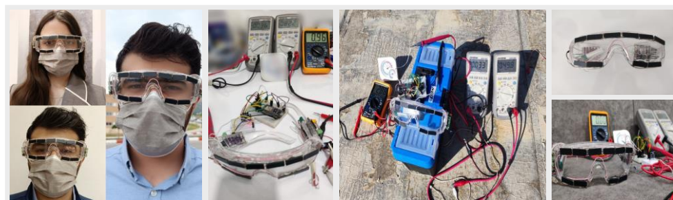
Figure 5. Hardware implementation of the prototype energy harvesting system on glasses as a wearable device, which are worn on the human body.
