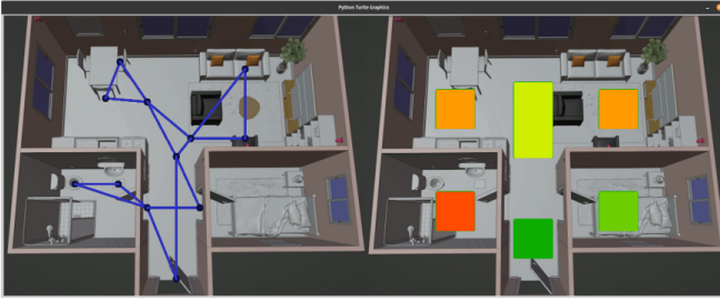
Fig. 5: Real-time visualization of in-home activity. Left: trajectory-based movement tracking reconstructed from consecutive ultrasonic sensor triggers. Right: zone-based residence-time heat map, where color intensity (green → yellow → orange → red) indicates increasing accumulated presence during the monitoring period.
