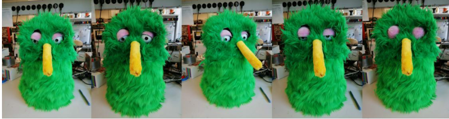
Fig. 2. Expressive states of the TUK robot used for neurofeedback. From left to right, the figure illustrates the five discrete expressive states corresponding to increasing EEG-derived attention levels: Angry (weak or poor signal), Sad (low attention), Neutral (neck and nose movement), Tired (slightly elevated attention), and Asleep (elevated attention). Each state is defined by a specific combination of eye position, eyelid closure, and nose orientation and is rendered through coordinated facial actuation.
