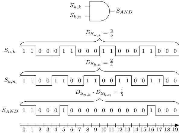
Fig. 5: Stochastic multiplication of two unary bit-streams using AND gate.  $S_{n,k}$  represents  $\frac{v}{n} = \frac{2}{5}$  with  $v = 2$  1s and a period of  $n = 5$  bits (Duty Cycle  $D_{S_{n,k}}=0.4$ ).  $S_{k,n}$  represents  $\frac{v}{k} = \frac{2}{4}$  with a period of  $k = 4$  bits (Duty Cycle  $D_{S_{k,n}}=0.5$ ). The output  $S_{AND}$  represents  $\frac{1}{5}$ .
