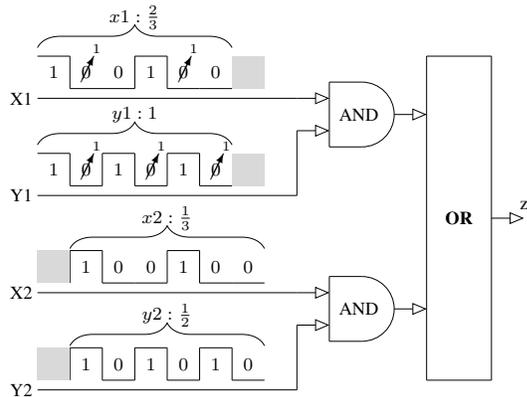
Fig. 4: The proposed MAC technique for four inputs, relative prime lengths  $n = k + 1 = 3$  and a relative delay between summands of 1 bit (marked by gray squares). The circuit is exact for inputs with at most 1 bit logic-1 per period (input values less than or equal  $\frac{v}{k} = \frac{1}{2}$ ). Because  $X1$  and  $Y1$  exceed this limit by  $c = 1$  bit, the result  $z$  has a maximum error of  $E_{upper} = 0.5$  (5).
