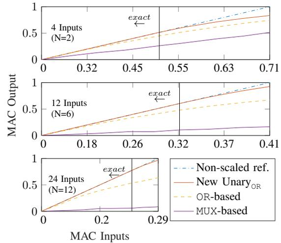
Fig. 7: MAC outputs for OR-based and MUX-based as well as the proposed  $\text{Unary}_{\text{OR}}$  as a function of input value and number of inputs. Up to the vertical line (thresholds from Table I), the proposed  $\text{Unary}_{\text{OR}}$  is exact and provides the same output as a non-scaled MAC, shown as diagonal line.
