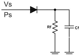
Fig. 5: Rectifying circuit and respective filter for the interpretation unit.
