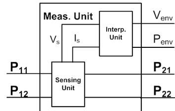
Fig. 3: Illustration of the measurement unit.
