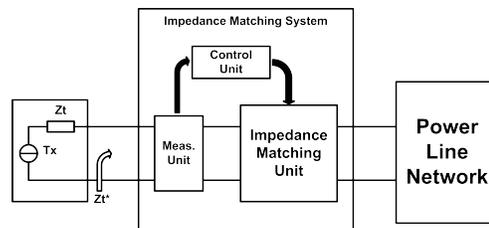
Fig. 1: Block diagram of an adaptive impedance matching system at the transmitter side.
