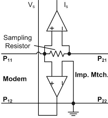
Fig. 4: Sensing unit circuitry including one resistor and two op-amps, connected to the modem at one end and to the Matching Unit on the other end.
