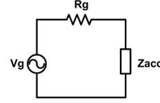
Fig. 6: Simplified matching problem where network impedance is modelled by  $Z_{acc}$ .
