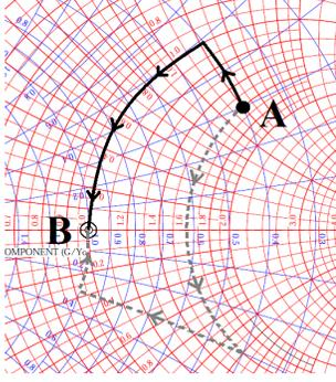
Fig. 2: Matching problem visualized in the Smith chart. Taking different paths from the given impedance point A to the desired impedance point B.
