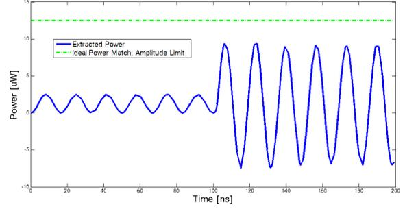
Fig. 8: Sample performance demonstration in the time domain. Transmission of power from source to the network ( $Z_{acc} = 1.8 \Omega$ ) before and after activating the adaptive impedance matching system at 100 ns.
