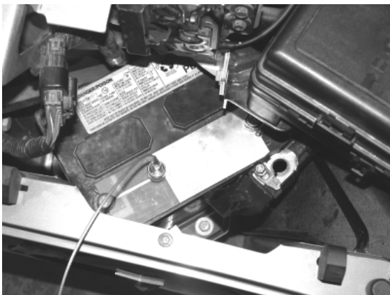
Figure 1. Microstrip interface PCB for 1-Port VNA measurements of the car battery.
